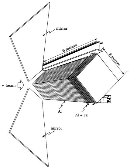
Fig. 1. Layout of the spark chambers of the CERN neutrino experiment (Aachen-Padova collaboration).
