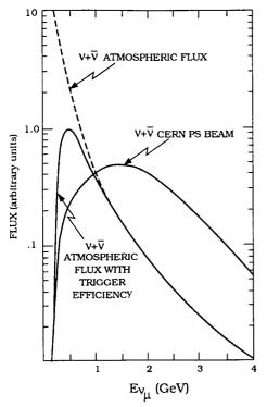
Fig. 2. Energy distribution for both the atmospheric neutrino flux at Fréjus and the CERN-PS neutrino beam.
