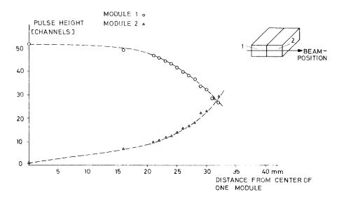
Fig. 6. The averaged pulse height of one module vs the beam position on the glass face for 1 GeV.
