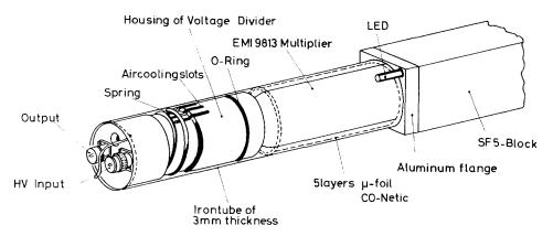
Fig. 2. Schematic drawing of a counter module.
