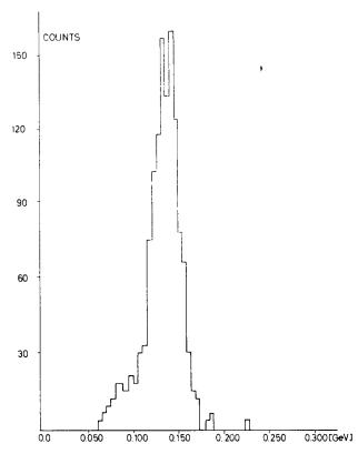
Fig. 7. The invariant mass plot of  $\gamma\gamma$  events in the reaction  $e+p{\rightarrow}e+\pi^0+X$ .
