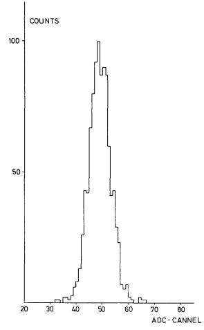
Fig. 4. The pulse height distribution for 1 GeV electrons.
