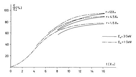
Fig. 1. The percentage of primary energy which is absorbed in a lead cylinder of radius r and length t (ref. 3).
