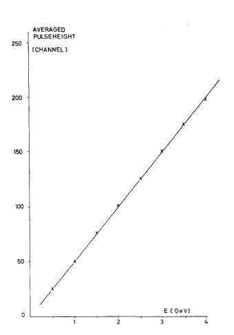
Fig. 3. The energy calibration. Averaged pulse height vs electron energy  $E_0$ .
