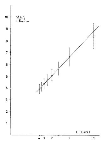
Fig. 5. The averaged energy resolution of all 182 elements vs  $1/\sqrt{E_0}$ . The bars indicate the spread of resolution among the 182 modules.
